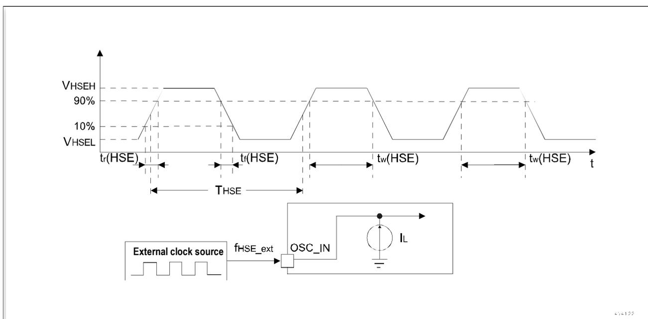
Figure 5-6 High-speed external clock source AC timing diagram
