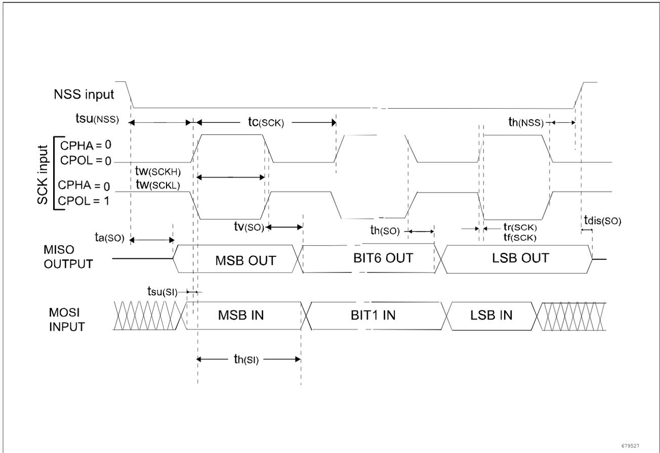
Figure 5-11 SPI timing diagram-slave mode and CPHA = 0, CPHASEL = 1
