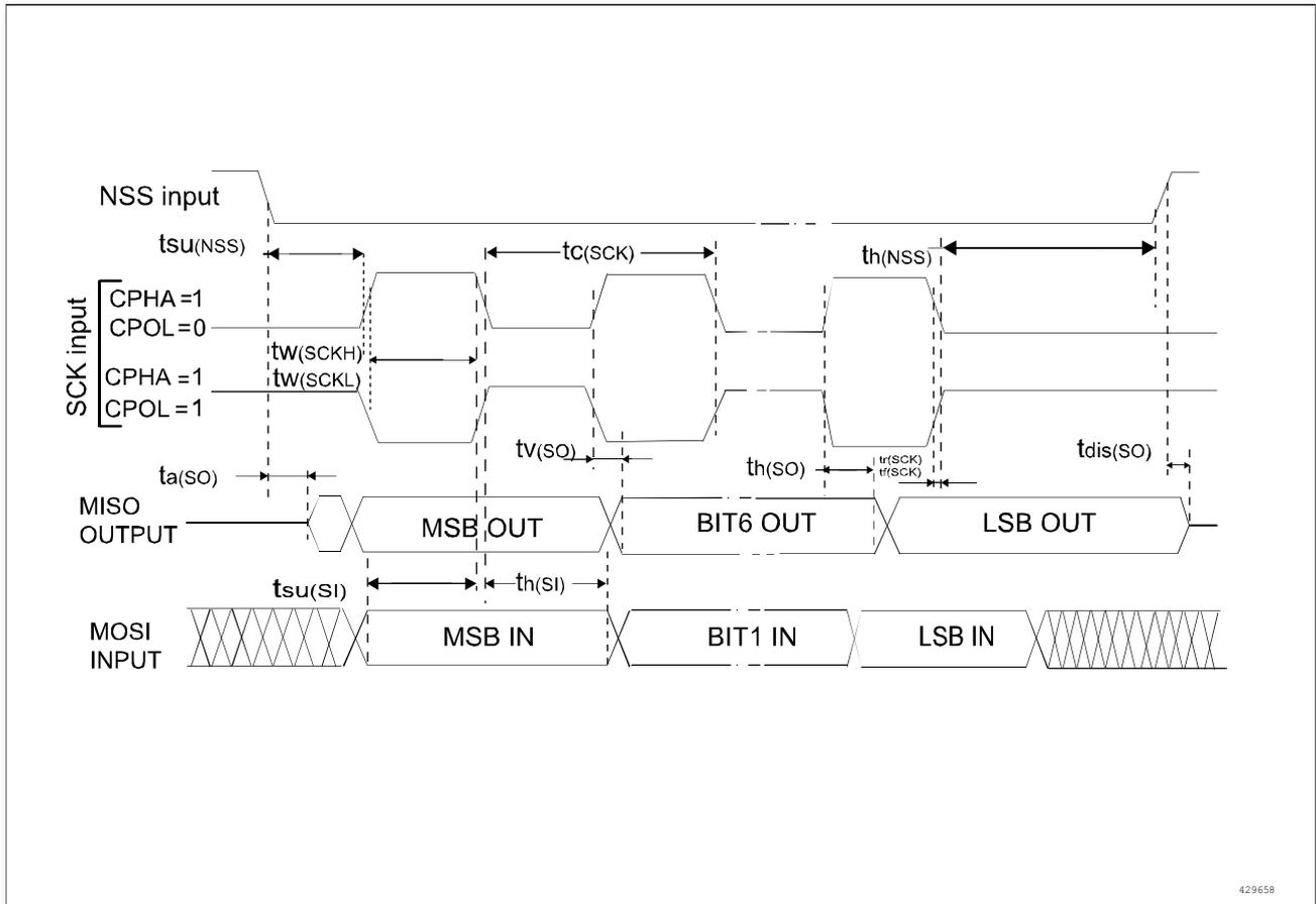
Figure 5-12 SPI timing diagram-slave mode and CPHA = 1, CPHASEL = 1 <sup>(1)</sup>
