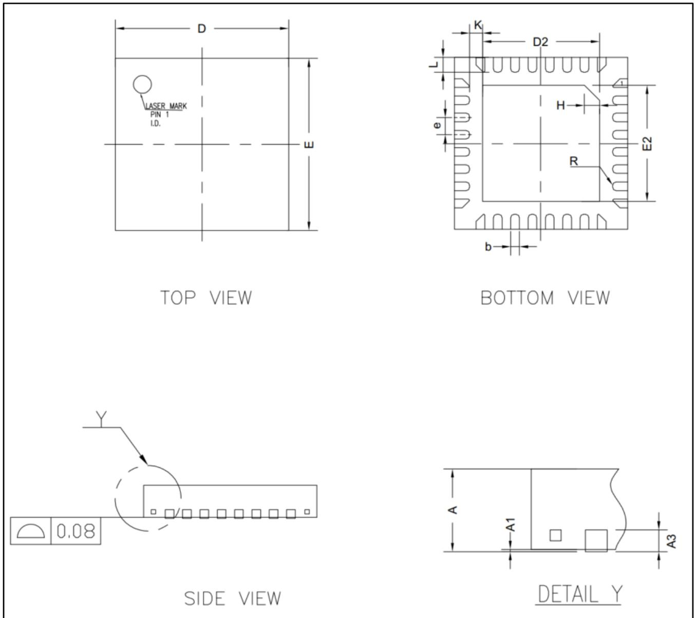
Figure 6-4 QFN32 4x4 mm<sup>2</sup> package dimension
