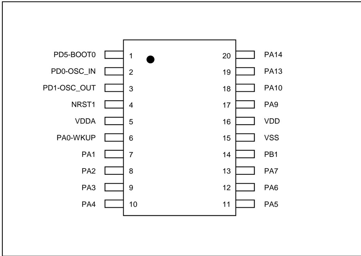
Figure 4-5 TSSOP20 pinout diagram
