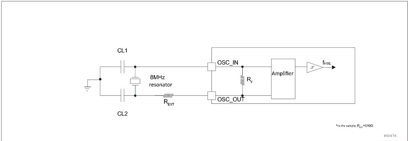
Figure 5-7 Typical application with an 8 MHz crystal
