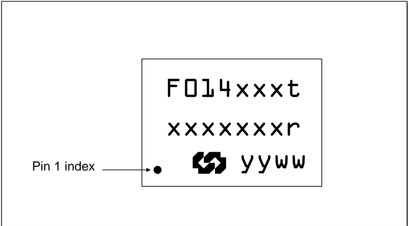
Figure 2-3 TSSOP20 package marking
