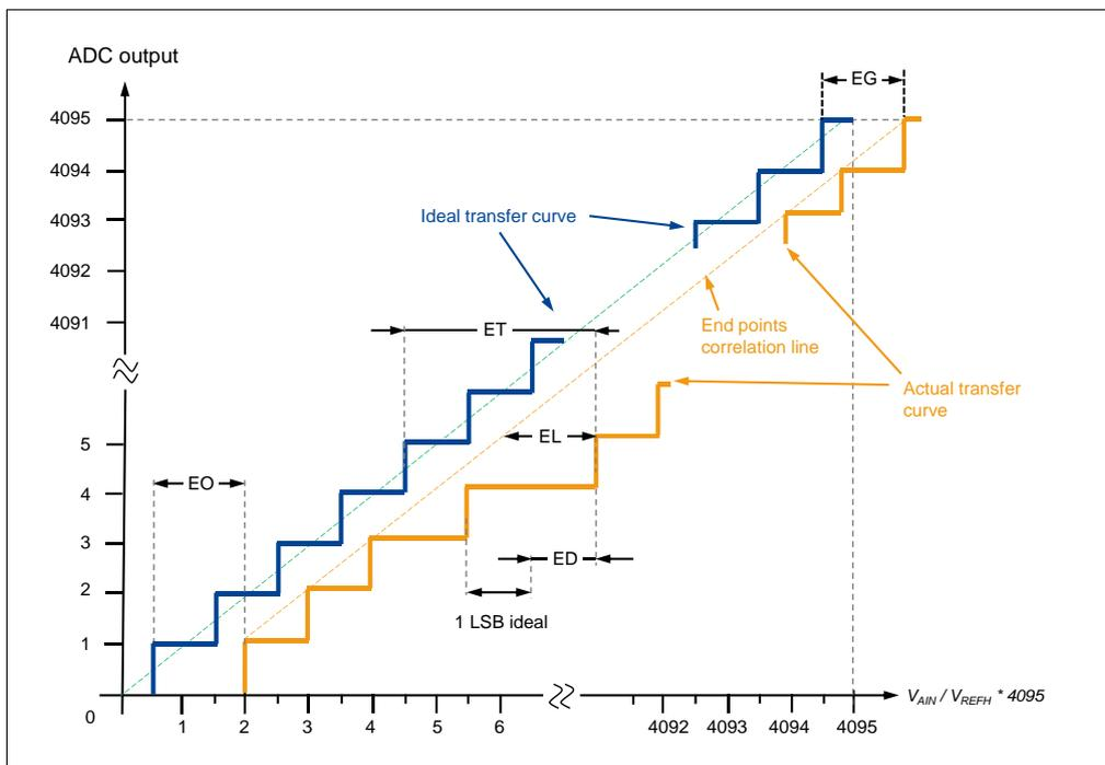
Figure 5-14 Schematic diagram of ADC static parameters
