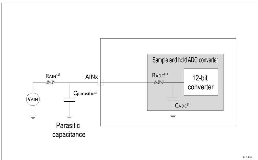
Figure 5-15 Typical connection diagram using the ADC
