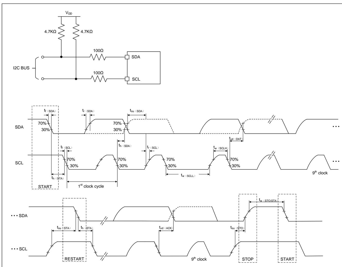
Figure 5-10 I2C bus AC waveform and measurement circuit (1)
