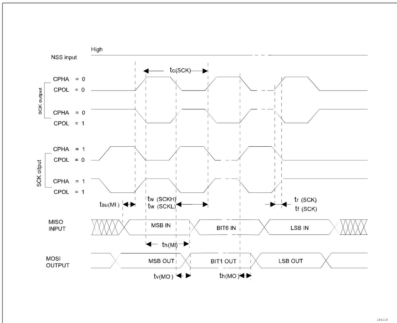
Figure 5-13 SPI timing diagram-master mode, CPHASEL = 1 <sup>(1)</sup>
