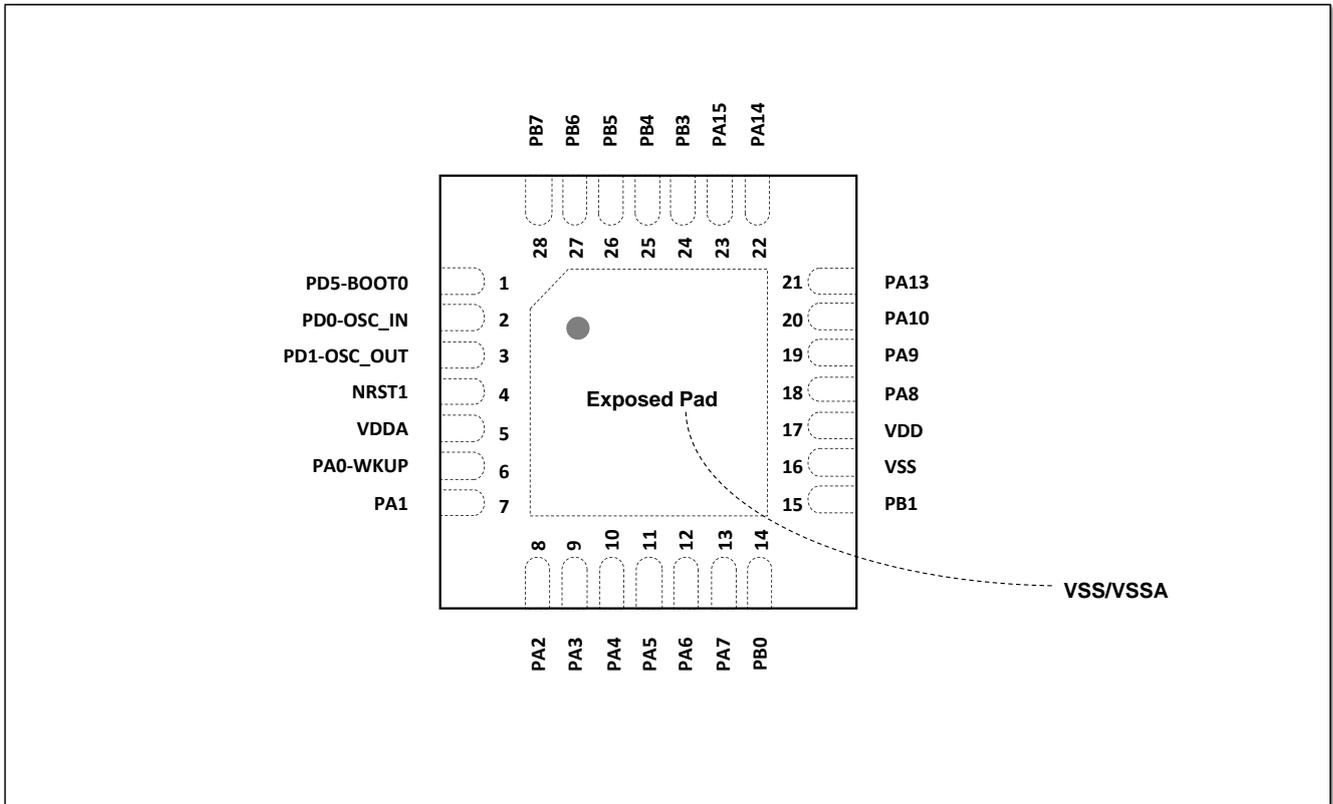
Figure 4-4 QFN28 pinout diagram
