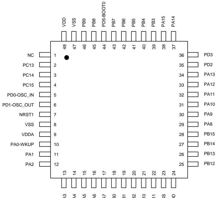
Figure 4-1 LQFP48 pinout diagram
