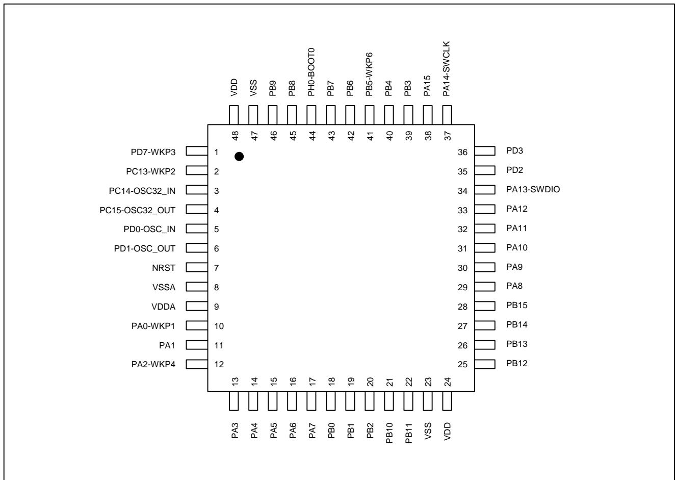
Figure 4-2 LQFP48 pinout diagram
